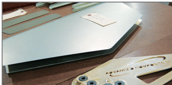
ACS helicopter fin (center) with a 3D printed drill guide (front).
