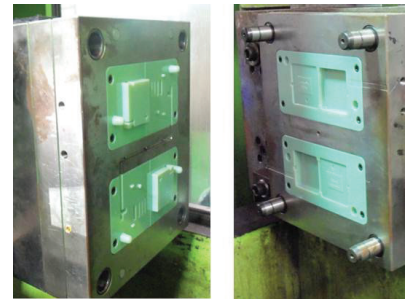
Figure 8 : PolyJet mold inserts on the molding machine. Left is the core and right is the cavity.
