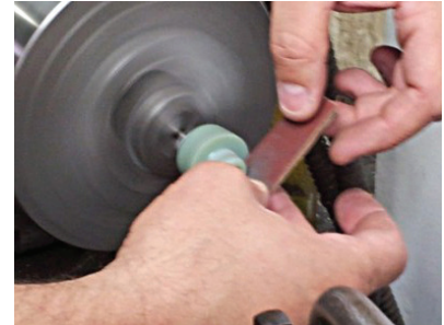
Figure 11: Finishing process of mold component.
