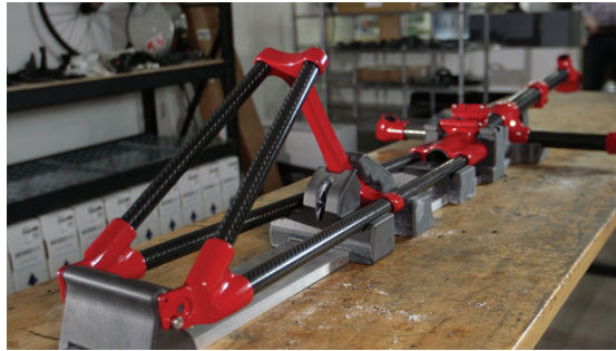
Figure 7: Utah Trikes uses FDM Nylon 12CF material in its advanced prototyping.
