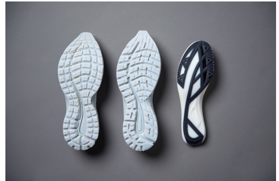
Figure 9: Brooks Running uses PolyJet technology to 3D print midsole and outsole prototypes to expedite its design process.
