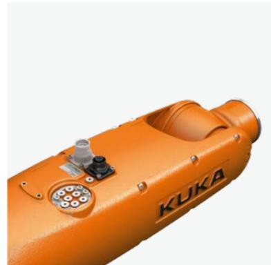
**Integrated energy supply system.** This is routed internally in the KUKA small robots, thereby saving space. It includes EtherCAT/ EtherNet (bus cable), three 5/2-way valves (compressed air), direct air line and inputs/outputs.
