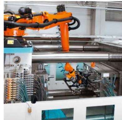
**In the system:** a space-saving KR AGILUS positions itself and accesses the assembly fixture from underneath
