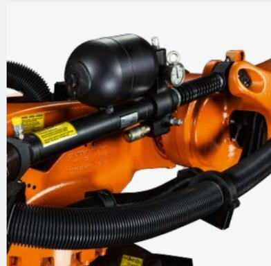
**Best performance with different payloads.** The hydropneumatic counterbalancing system allows for infinitely variable – and therefore optimal – adaptation of the restoring forces to the masses moved. It ensures outstanding dynamic performance and maximizes the energy efficiency of the robots at the same time.
