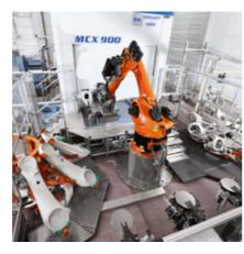
Reliable, even with heavy components Even heavy components are loaded precisely, with no risk of damage to the machine or clamping equipment. The machine is loaded with pin-point accuracy, ruling out the possibility of rejects due to incorrect positioning.
