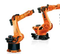
For heavy loads up to 1.3 tonnes KUKA robots are ideally compatible with machine tools and command an extremely large work envelope.
