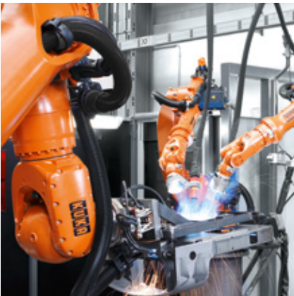
Jigless welding in commercial vehicle production: the handling robot positions the workpiece to be welded for the two welding robots.
