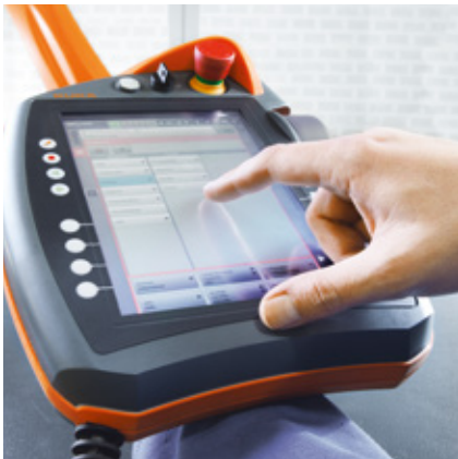
Antireflection touch display Operator control is quick and easy via the well-lit 8.4" screen with an intuitive user interface. Safe and quick operation is even possible when wearing protective gloves.
