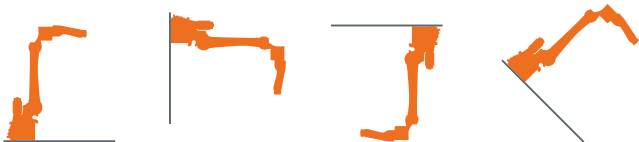
Flexible mounting options Flexible cell design thanks to floor, ceiling, wall or angle-mounted positions. Increased accessibility thanks to the CYBERTECH series' optimal use of space.
