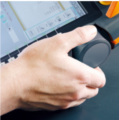
6D mouse and motion keys With the intuitive 6D mouse, the robot can be moved in all directions as if the welding torch were being guided manually – without the need for repositioning. The 6D mouse can also be used in combination with the motion keys to make quick and targeted settings.
