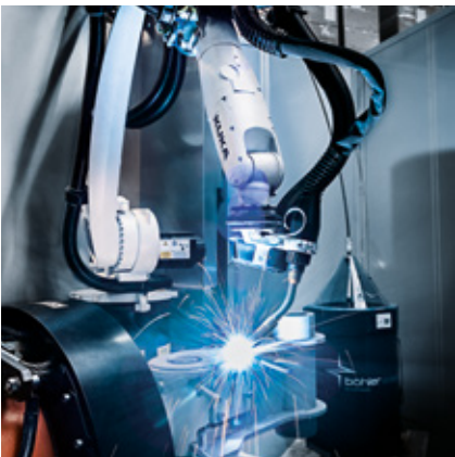
Welding of an articulated lever (concrete pump truck)
