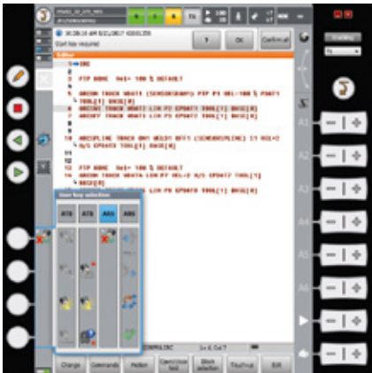
Status keys The status display offers the controls required during programming and production. The available functions include the following: • Welding • Wire feeding • Gas • Acknowledgement of power source messages
