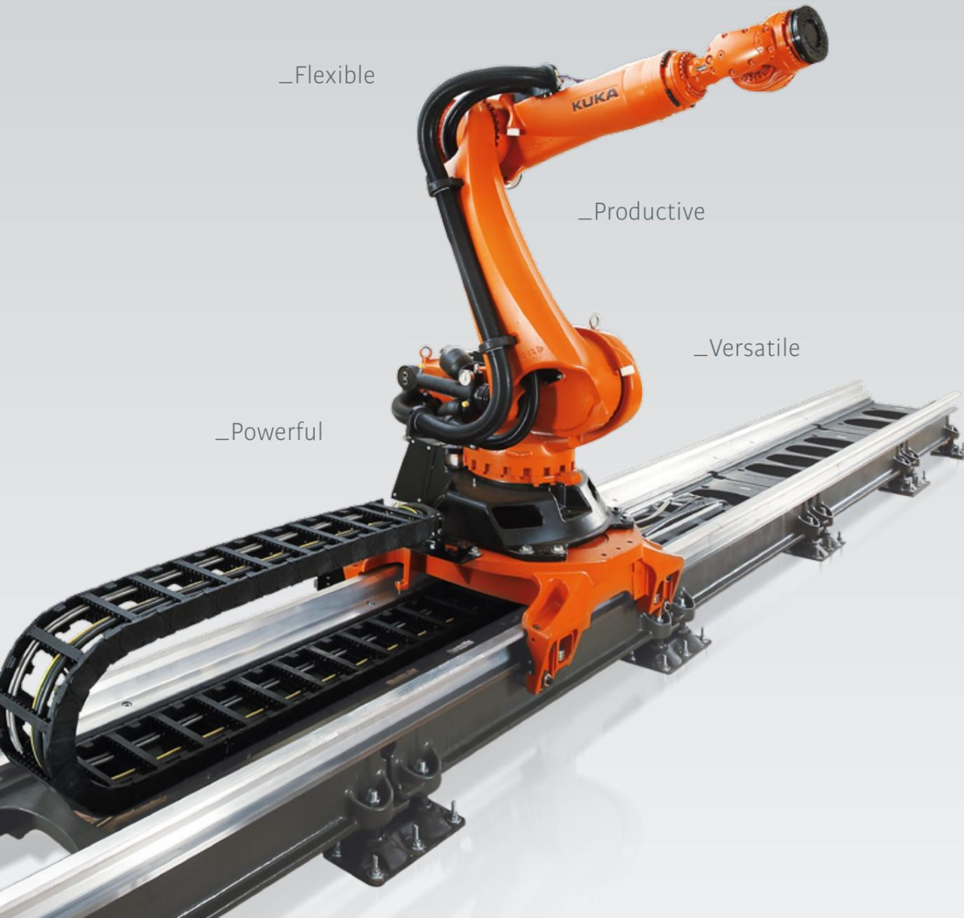
**Positionally accurate.** Up to four robots can be operated on one linear axis. Multiple robot positions on the linear axis allow optimal adaptation to existing requirements and workspaces.
