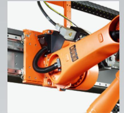
KUKA gantry robots can be installed in an inverted or side-mounted position – meaning they can be deployed flexibly.
