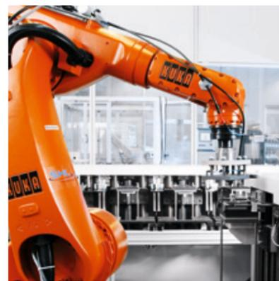
Loading of injection molding machines with stamping grids in order to manufacture control casings for the automotive industry
