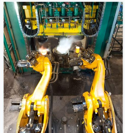
**Light exercise:** The KR 1000 titan F unloads steel blanks weighing up to 400 kg with a consistently high cycle time and without breaking into a sweat – even in the case of forged parts with a temperature of 1200 °C.
