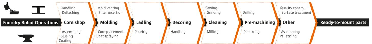
Example of a process chain from the molten metal through to the ready-to-install part in the sand mold.
